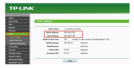
• The subnet mask of the NVR must be the same as the subnet mask in LAN port status. The default gateway of the NVR is the same as the IP address in LAN port status. The primary DNS and secondary DNS can be the same as the DNS in WAN port status.
