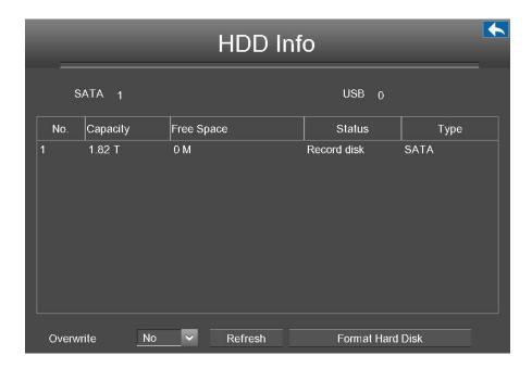
[Overwrite]: When the HDD is full. You can select the whether cover the earliest recording. Select Yes, the NVR will cycle cover the earliest recording; Select No, the NVR will stop recording.
