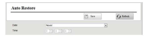
You can configure the Date and Time. The NVR system will be maintained at the setting time.
