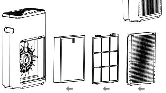
Note: There are internal and external points, the one with the pull tab facing out; be sure to install the front panel before use.
