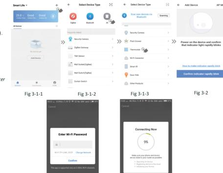
This is EZ mode which provides fast network connection between your app and your device. If your router doesn't support it or your wifi signal is weak or you can not connect by EZ mode, press the AP Mode
